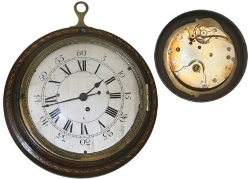
Figure 1: The Sedan clock with (top right) its 'pocket watch' movement
